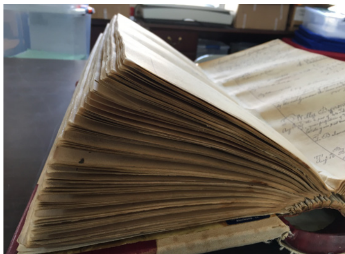
Sussex County Guardians Accounts, 1754-1789, was cellulose acetate laminated in 1939 and the pages are chipping and breaking, stiff, splitting and warping, with heavy burn through.
